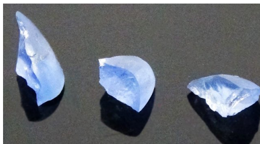
Stress tested (via hammer impact) HPHT sapphire fragments reveal newly-formed cracks radiating toward center.
