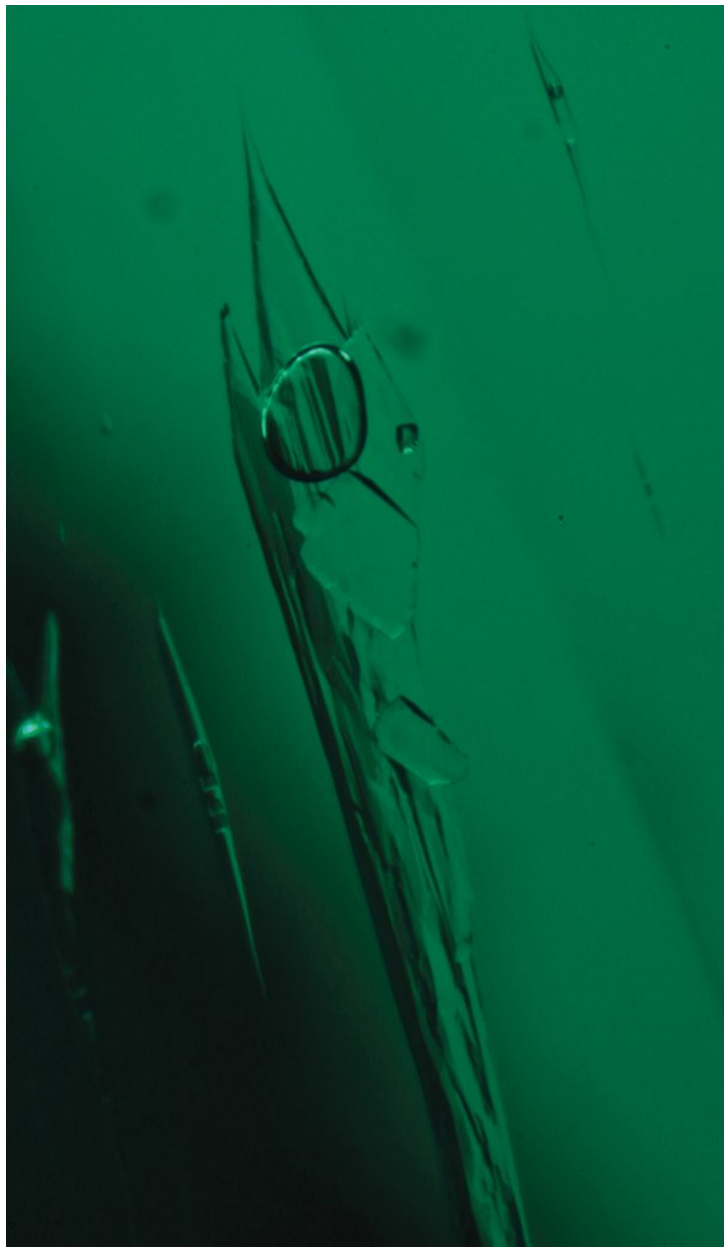
A 3-phase (liquid, solid, vapor) inclusion typically found in a Colombian emeralds.
