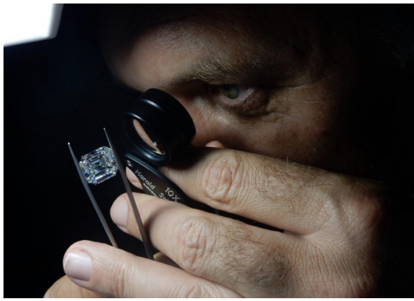
Fig. 9: The faceted 10.02 ct gem-quality E color and VS1 synthetic diamond is featured here with CGL-GRS's Branko Deljanin. The dimensions are 12.49 x 12.43 x 7.37 mm. The clarity of VS1 and the color of E is combined with a very good polish and symmetry and an excellent cut (reminiscent of Asscher cut). The NDT's "landmark" synthetic diamond is believed to be one of the largest of its kind in the world, and according to our best knowledge, sets the new world record for a faceted synthetic diamond of this quality. The stone was available at MGJ Conference 2015 in Athens (Greece). Photo by John Chapman.
