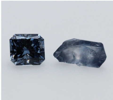
Fig. 7a: Two synthetic fancy blue diamonds, produced by HPHT (NDT). The left is a faceted synthetic of 0.56ct (VS2 clarity) and on the right a crystal of 0.67ct. Both are type IIb synthetic diamonds (both stones part of GRS reference collection). Photo by Matthias Alessandri.
