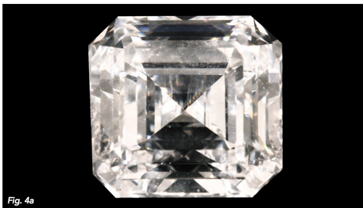
Fig. 4a: The faceted 10.02ct (E, VS1) synthetic diamond by NDT is according to our knowledge the new world record for a gem-quality faceted synthetic diamond in terms of size.
