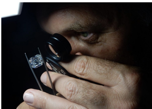
Fig. 9: The faceted 10.02 ct gem-quality E color and VS1 synthetic diamond is featured here with CGL-GRS's Branko Deljanin. The dimensions are 12.49 x 12.43 x 7.37 mm. The clarity of VS1 and the color of E is combined with a very good polish and symmetry and an excellent cut (reminiscent of Asscher cut). The NDT's "landmark" synthetic diamond is believed to be one of the largest of its kind in the world, and according to our best knowledge, sets the new world record for a faceted synthetic diamond of this quality. The stone was available at MGJ Conference 2015 in Athens (Greece). Photo by John Chapman.
