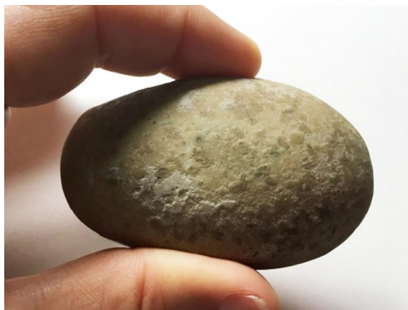
Figure 3: Tumbled and chemically altered surface of synthetic aggregate. Photo: A. Peretti, © GRS Gemresearch Swisslab AG.
