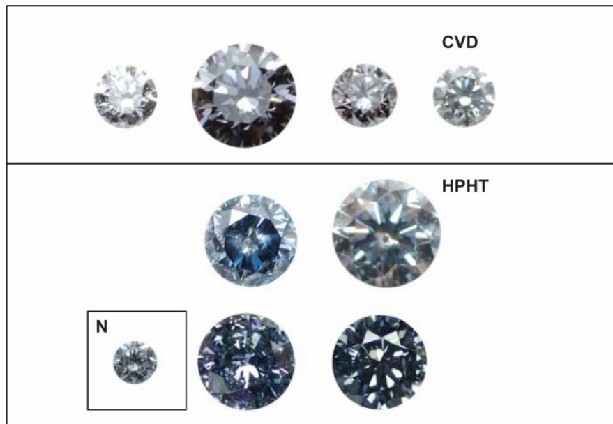
4 CVD-grown diamonds from Orion PDC (top) in colour ranging from Fancy light blue to Fancy greyish blue, weighing from 0.30 - 0.65cts respectively. 4 Synthetic HPHT-grown diamonds from Chatham, AOTC, TAIRUS (bottom) plus one natural blue diamond (insert) from GRS-CGL reference collection for this research.
