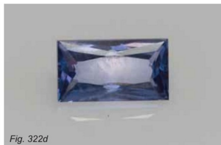
Fig. 322a-d: Spinel produced by flux (pulled method) of different colors, including pinkish-red, lavender, color-changing and violetish-blue color varieties. Synthetic spinels cut by GRS from the rough, over 1ct each in size.
