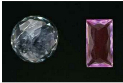
Fig. 325: Two synthetic spinels as seen through a polariscope with crossed polarizers. Left a Verneuil synthetic spinel and on the right the new type of synthetic spinel produced from flux. Note only the Verneuil spinel shows cross-hatched anomalous interference patterns.
