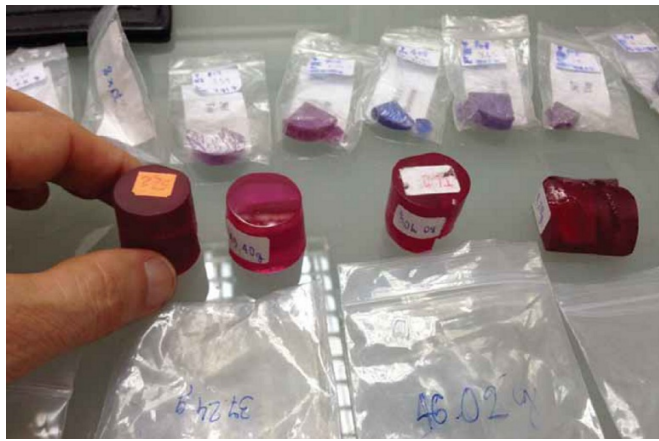
Fig. 320: Spinel commercially produced by the pulled method from flux. Note the approximate 5cm diameter of the cylinders and the different color varieties. The rough is about 250ct in size. Photo by AP at Tairus, Bangkok.
