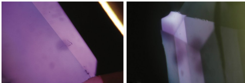
Fig. 2b Surface staining in a Co-diffusion treated spinel. It is located at feathers and cracks on the surface. The spinel was repolished after diffusion-treatment but these features were not removed.
