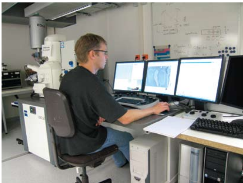
Fig. Tan66 The SEM instrument and operation console of the University of Berne, Earth Science Department, Switzerland. To the left details of the SEM (Zeiss EVO 50): An opened sample chamber, surrounded by a variety of detectors, such as Secondary Electron Detector (SE), Backscattered Electron Detector (BSD) and an X-Ray Detector (EDX) with a Polymer Window (S-UTW) for micro-chemical analysis. To the right the SEM (Zeiss EVO 50 equipped with SmartSEM acquisition software) operated by Dr. Marco Herwegh and one of the authors (WB).
