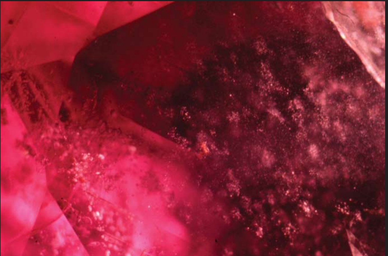
Fig. Tan113 Micro-particle inclusions resembling “Snow Flakes”. Fiber-optic illumination. Sample No. GRS-Ref7861b.
