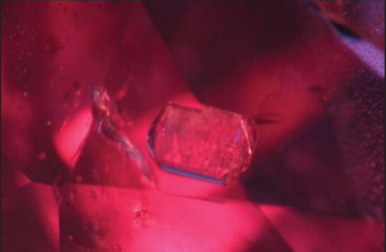
Fig. Tan58 Xenothim inclusion in a Winza ruby is shown (Identification by ED-XRF micro-analysis). Crystal size is over 1mm. Fiber optic illumination. 15x magnification. Sample No. GRS-Ref7861c.
