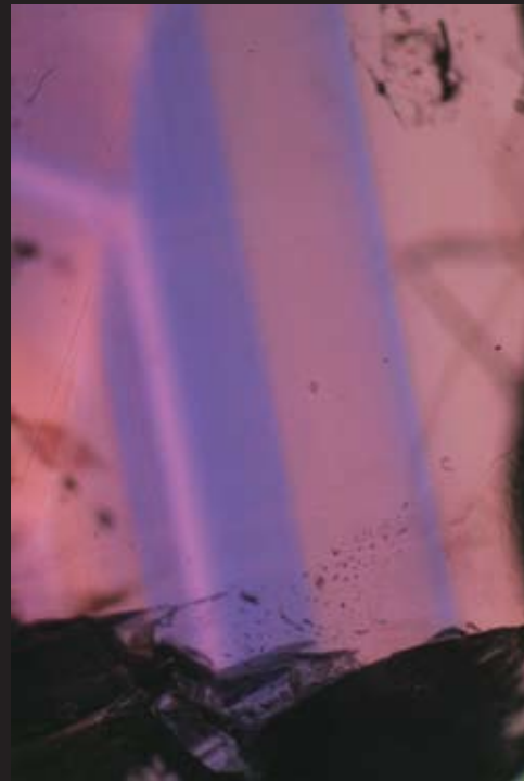
Fig. Tan84a, b Micro-photo with detail on growth structures is shown in reflected light. The lightening did enhance the presence of micro particles in the Winza ruby. A white line became visible of the shape of “Sky scrapers” (S, Fig. Tan84a). A picture in the transmitted light made the color oscillations visible that occur in addition to the presence of micro-particles (Fig. Tan84b). Sample No. GRS-Ref7152.
