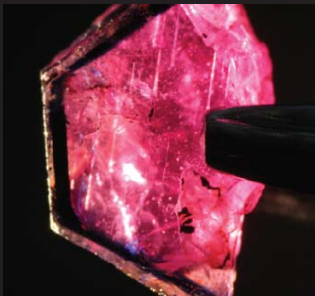
Fig. Tan94a, b Two examples of rough ruby crystals are shown (view in direction of the c-axis). The pinkish-red core is followed by a layer of blue color in the mantle of the crystal. The outermost layer consists of a milky-white rim. (Right) Sample No GRS-Ref7484 (Tan39), weight 4.13ct.
