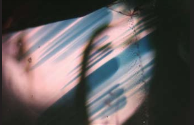
Fig. Tan106 Blue color zoning in a cabochon ruby that appears like a series of discs. Note: the presence of a fluid feather in a direction perpendicular to this color zoning. Sample No GRS-Ref8313.
