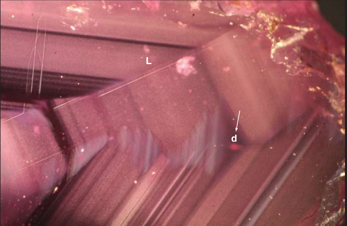
Fig. Tan83 Cross section parallel to the c-axis of a Winza ruby (slightly rotated along the c-axis in comparison to Fig. Tan82). This crystal termination feature appeared and disappeared during crystal growth (d). Occasionally forming triangular patterns in the ruby (see arrow). Picture in reflected fiber optic light that enhanced the presence of micro particles. In direction of the c-axis a whitish line was present in the ruby (L). Sample No. GRS-Ref7152.
