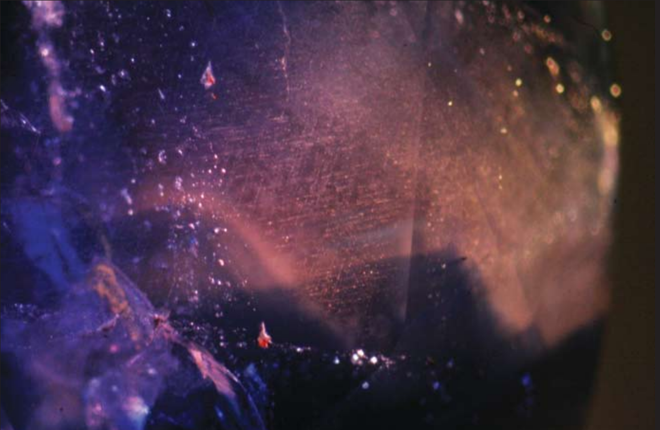
Fig. Tan119 Oriented pinpoints in a faceted sapphire. A color whole is present in the sapphire and pin point rutile particles are present in the typical crystallographic orientation inside the color window. No long rutile needles were found. Fiber-optic illumination. Sample No. GRS-Ref8195.
