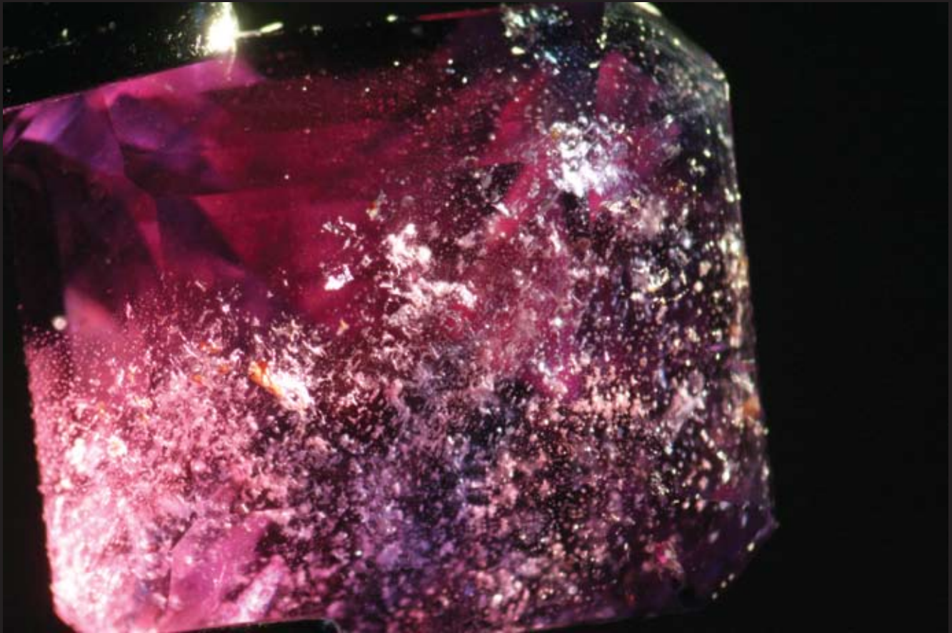
Fig. Tan37 Photo of a faceted purplish-red ruby from Winza with numerous fluid inclusions. The fluid inclusions are entirely filled with whitish daughter minerals. Sample No. GRS-Ref7125. Fiber optic and transmitted light.
