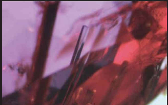
Fig. Tan46 A series of pargasite in a Winza ruby (Transmitted light 40x magnification, White field illumination, Sample No. GRS-Ref7814).
