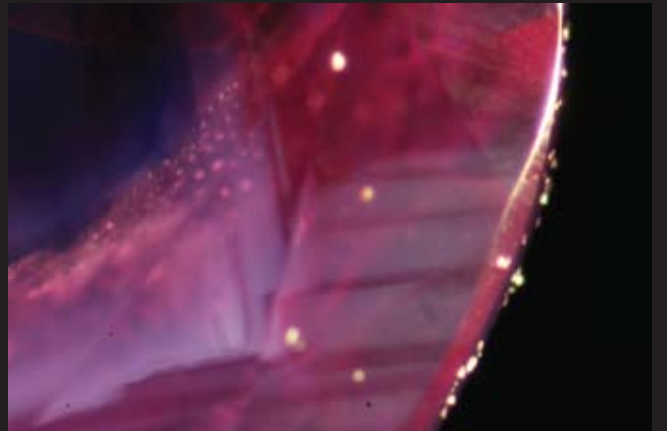
Fig. Tan108 Blocks of white color zones adjacent to an intense blue color zone in a faceted ruby from Winza. In the transition zone between the blue and milky zone is a fluid feather. Sample No. GRS-Ref A.
