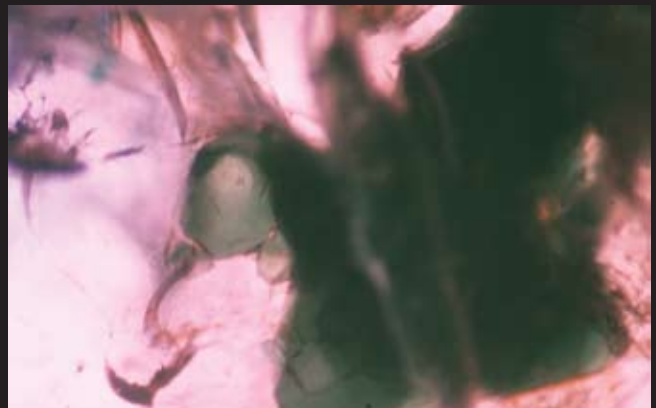
Fig. Tan47 A flat void in a Winza ruby is filled with an aggregate of pargasite. The Cl-pargasite is chemically zoned with more intense colored rims. (Sample No. GRS-Ref1379)
