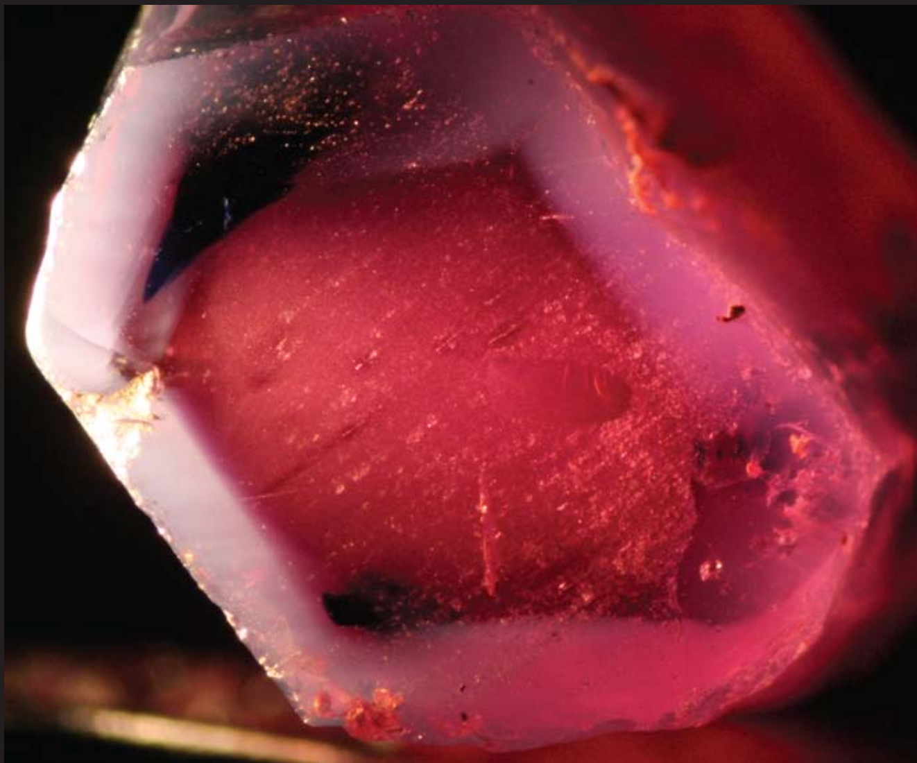
Fig. Tan93 A rough “Winza” ruby has been cut perpendicular to the c-axis. The ruby is composed of a red core and a milky rim. Every second corner, a blue triangular color zone is found parallel to rhombohedra growth faces. Sample No GRS-Ref Tan22.
