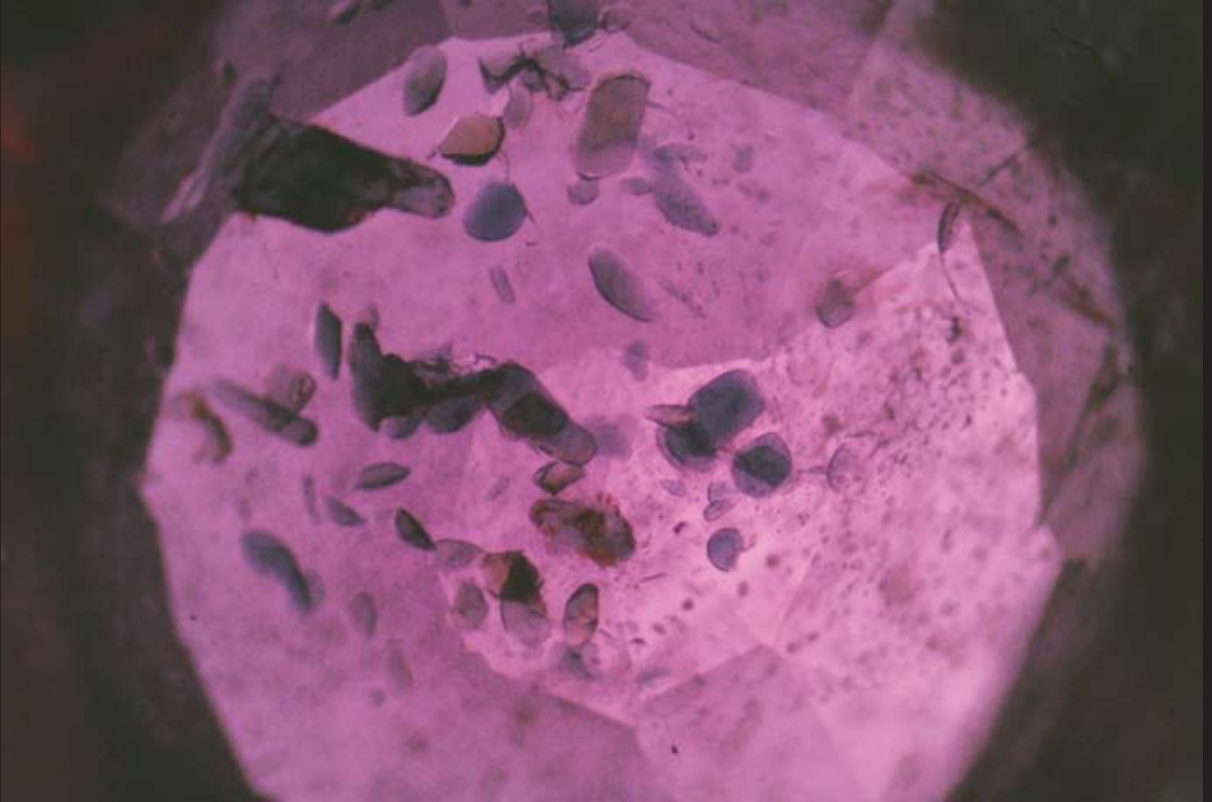
Fig. Tan48 Pargasite inclusions in a Winza pink sapphire. Different colors of the pargasite inclusions are due to different orientation of the minerals (strong dichroism) and/or variations in its chemical composition.
