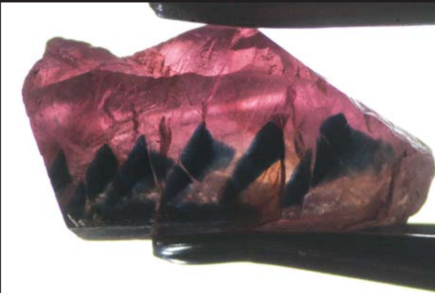
Fig. Tan91 Winza ruby rough with two polished windows is shown. Two different type of blue color zoning are found in this crystal. A series of triangular blue color zones resembling “shark teeth patterns”, are arranged along the c-axis and an outer blue zone, which is formed parallel to a steep pyramid in the ruby. Sample No. GRS-Ref7557, weight 3.14ct, length 10.5mm.
