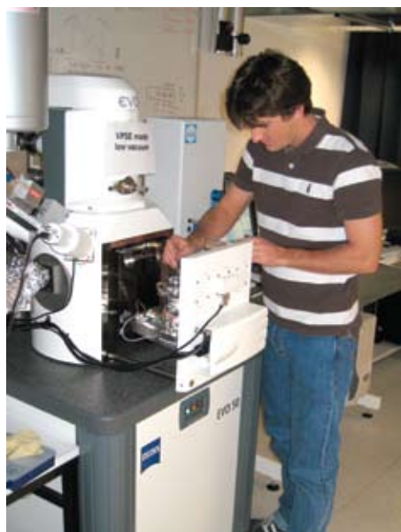
Fig. Tan66 The SEM instrument and operation console of the University of Berne, Earth Science Department, Switzerland. To the left details of the SEM (Zeiss EVO 50): An opened sample chamber, surrounded by a variety of detectors, such as Secondary Electron Detector (SE), Backscattered Electron Detector (BSD) and an X-Ray Detector (EDX) with a Polymer Window (S-UTW) for micro-chemical analysis. To the right the SEM (Zeiss EVO 50 equipped with SmartSEM acquisition software) operated by Dr. Marco Herwegh and one of the authors (WB).
