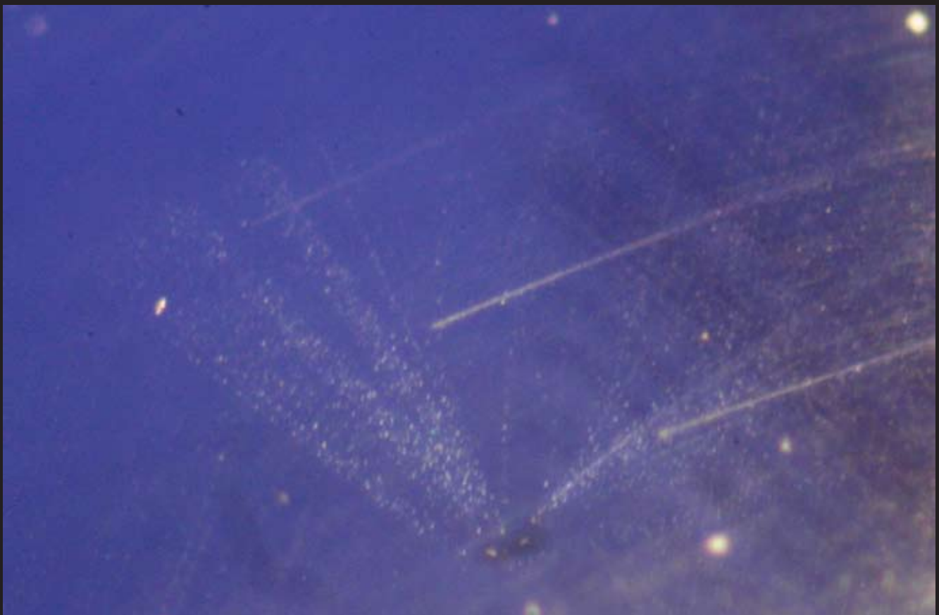
Fig. Tan115 A “comet tail” is formed at the surface of an opaque inclusion. Fiber-optic illumination, 60x magnification.
