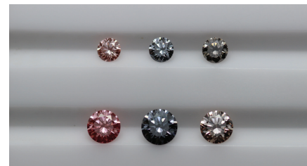
Fig 14: Group of PDC Orion pink and blue, Scio Diamonds brown CVD grown diamonds. Courtesy of GRS, Hong Kong
