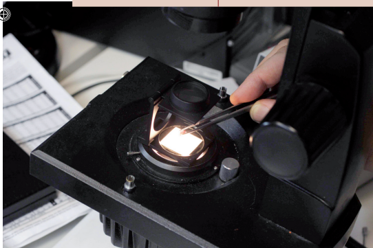
Fig 13: Pink diamond of unknown origin between cross polarized filters under the microscope. Courtesy of CGL-GRS, Vancouver.
