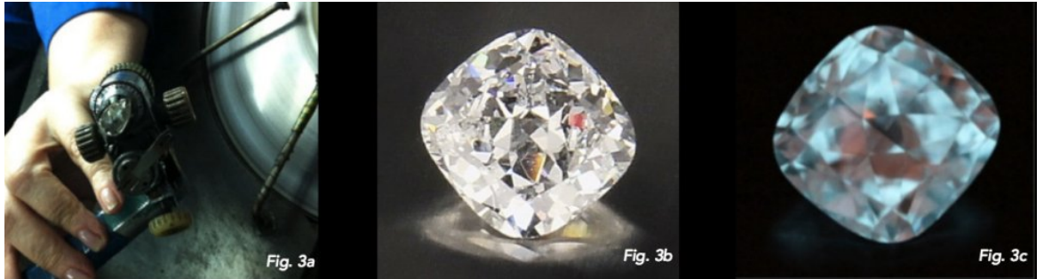
Fig. 3a: NDT synthetic grown diamonds are synthesized and polished at their facility in St. Petersburg. In the picture is a 5.13 ct pear shaped lab-grown diamond on the polishing wheel at NDT in-house cutting factory. Photo by Branko Deljanin. Fig. 3b: icture shows a HPHT-grown cushion shaped diamond (4.30ct, D color, VS2) by NDT. Photo by NDT. Fig. 3c: Same HPHT grown diamond as in Fig. 3b, after exposure to pinpoint-light shows bluish orange luminescence and orange phosphorescence in darkened room. Photo by Mikko Åström.
