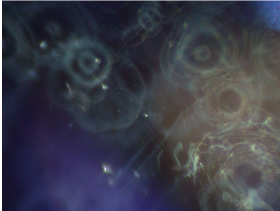
Circular inclusions resembling "fish eggs" found in a Beryllium-treated blue sapphire.
