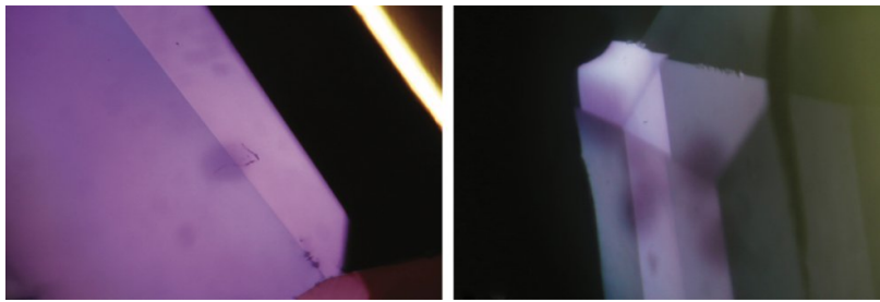
Fig. 2b Surface staining in a Co-diffusion treated spinel. It is located at feathers and cracks on the surface. The spinel was repolished after diffusion-treatment but these features were not removed.
